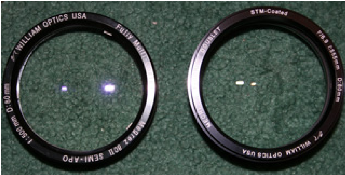
The 'supercoated' lens (right) reflects much less light than the 'Fully multicoated' lens (left)
